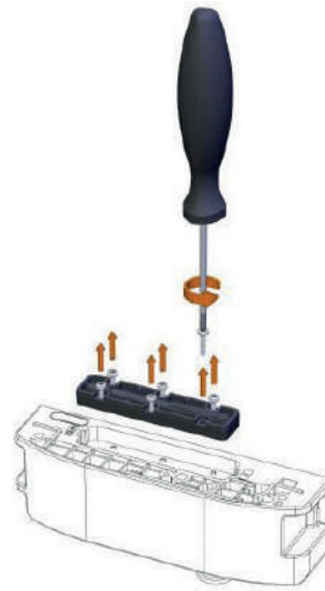
Phase 2. Unscrew the 6 fixing screws and lift the plate
