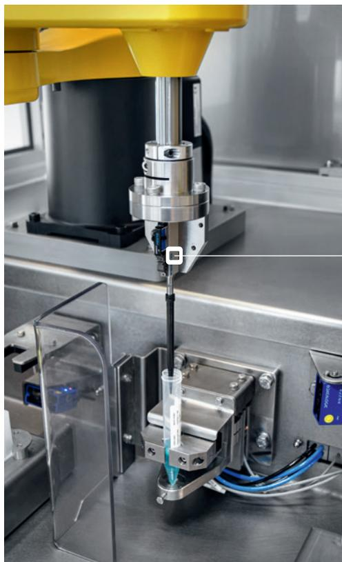
**Extremely small pipetting volumes:** the second robot arm with the pipette head distributes liquids onto a microwell plate.
