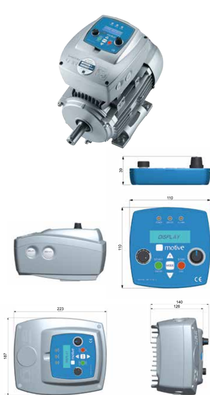
DIMENSIONS of NEO-WIFI-3 and KEYPAD
