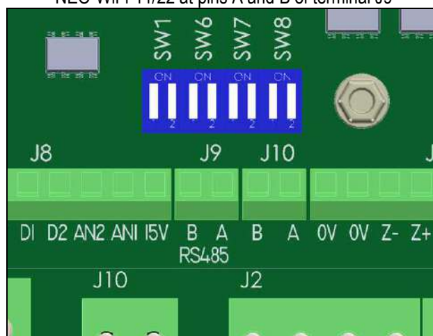
NEO-WiFi-11/22 at pins A and B of terminal J9
