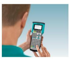
Easy operation via the practical keypad: the THERMOMARK GO.K input field prioritizes frequently used characters and offers a large selection of special characters as well as eight bar code types.
