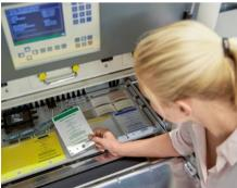
To simulate several years of use outdoors, in our laboratory the marking materials are exposed to cyclical stresses through UV radiation and humidity, and are thus tested in accordance with DIN EN ISO 4892-2.
