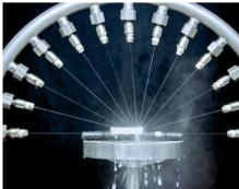
The IP degree of protection of markings is determined with the help of a water jet test and indicates the material's scope of protection against the ingress of foreign bodies as well as the tightness of seal against moisture.
