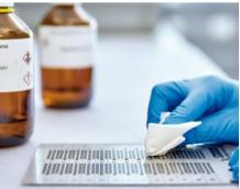
Aggressive cleaning agents can corrode the markings and cause the material to fade, the text to become illegible, or result in brittle fractures. Marking materials must therefore have a high resistance to chemicals.
